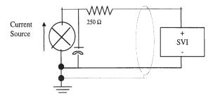
Figure 27. Resistor Add in Series with Current Source
