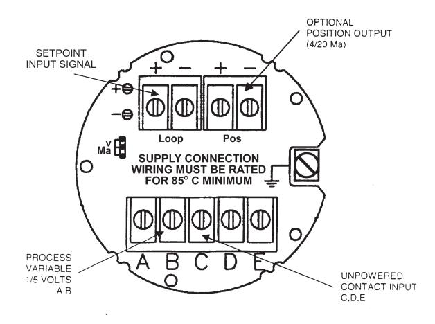
Figure 24a. Electrical Connections to Main Terminal Board
