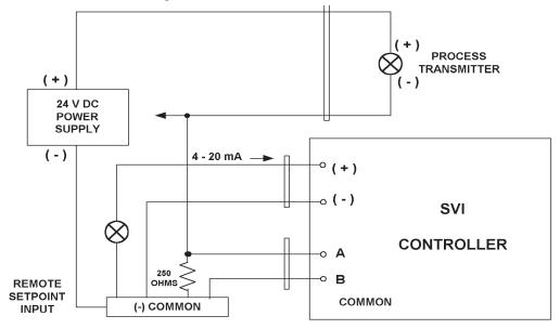
Figure 8. Single Loop PID Configuration with Process Feedback
