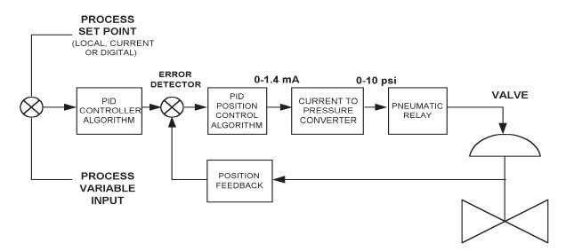
Figure 3. Block Diagram of SVI Controller/Positioner
