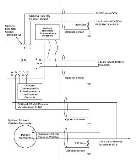
Figure 24b. General Area Purpose Installation
