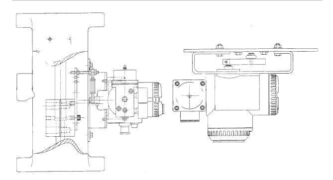
Figure 21. Typical SVI Mounting on 84/85 Actuator
