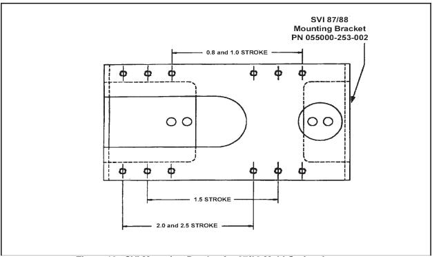
Figure 18. SVI Mounting Bracket for 87/88 Multi-Spring Actuator
