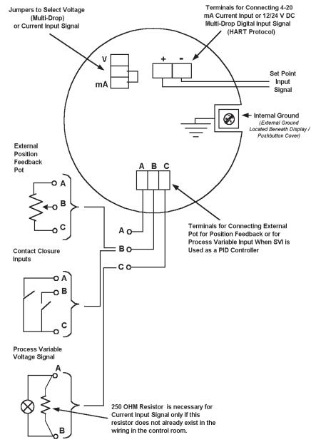
Figure 44. Wiring Connections
