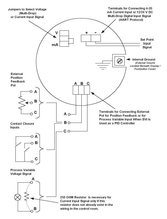
Figure 24. Electrical Connections to Main Terminal Board (Current Production)
