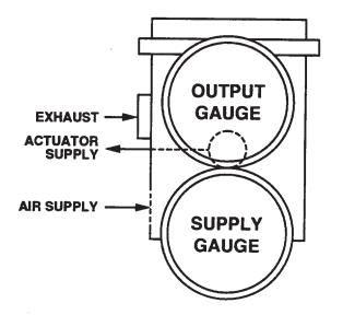
Figure 43. Exhaust, Actuator and Air Supply Connections
