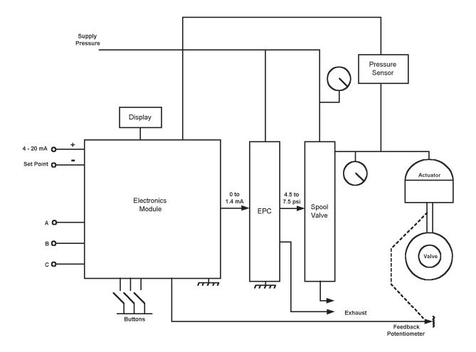
Figure 3a. SVI Block Diagram
