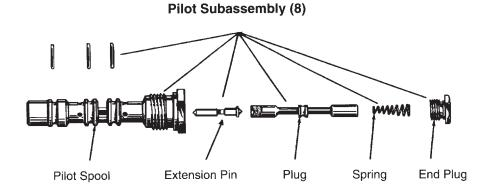
Figure 45. Pilot Subassembly
