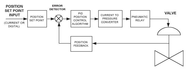
Figure 2. Block Diagram of SVI Positioner
