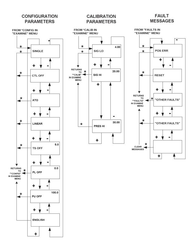
Figure 35. Parameter and Message Displays
