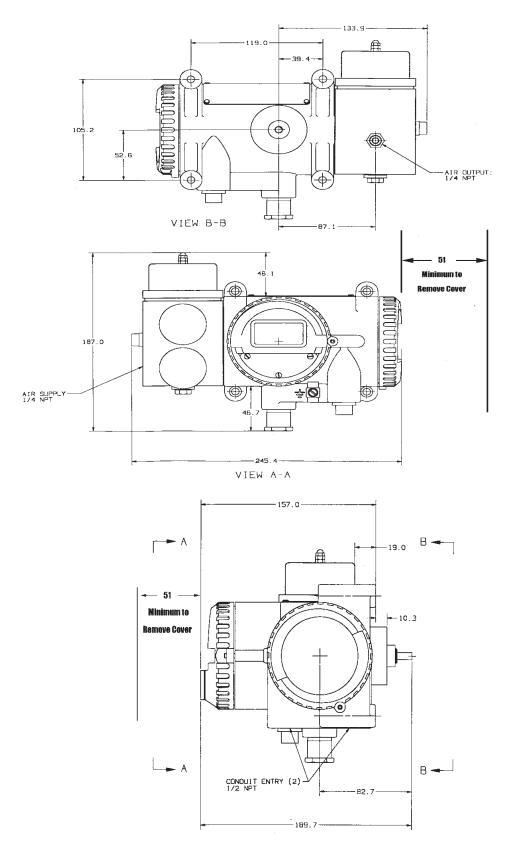
Figure 21a. Smart Valve Interface Outline Drawing
