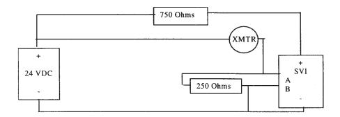
Figure 10. Local Set with Voltage Source
