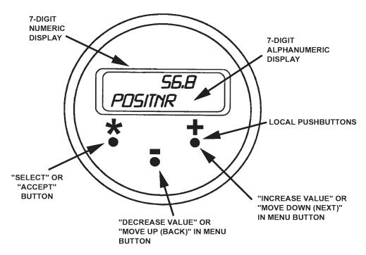
Figure 36. Local Display and Pushbuttons
