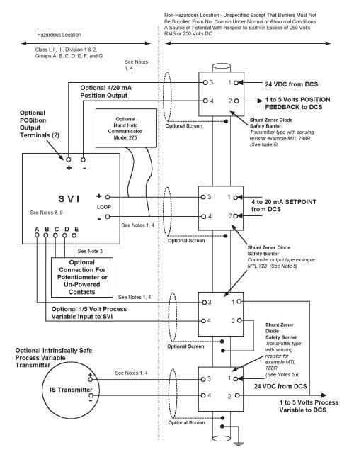
Figure 25. Approved Intrinsically Safe Installation Control Drawing
