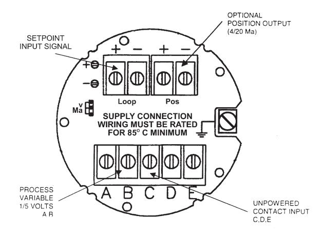
Figure 44a. Wiring Connections - 1999 Release
