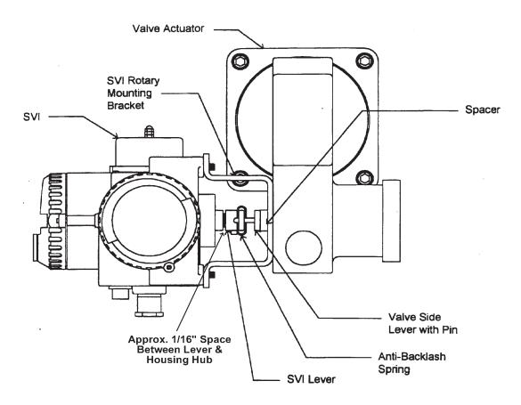
Figure 15. SVI Mounting on Rotary Valves
