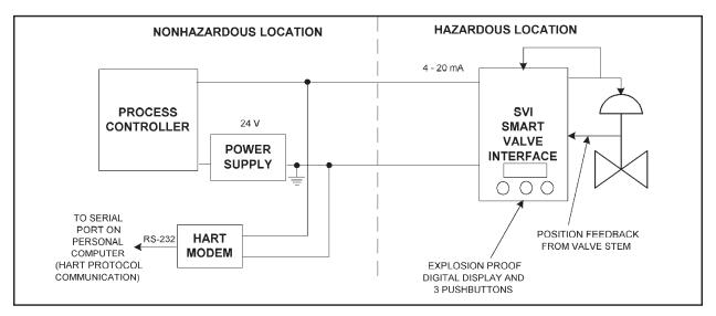
Figure 6. System Diagram – Explosionproof (Flameproof) Installation
