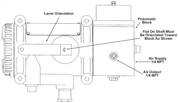
Figure 14. Orientation of SVI Lever and SVI Shaft
