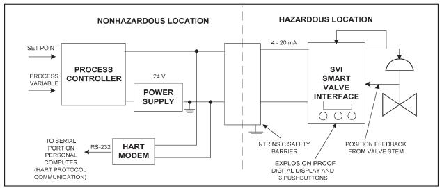
Figure 5. System Diagram – Intrinsically Safe Installation
