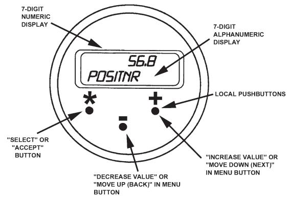
Figure 30. Local Display and Pushbuttons
