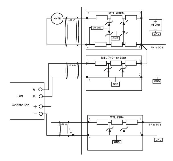
Figure 9. Intrinsically Safe Single Loop PID Configuration
