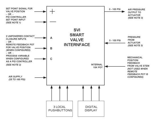
Figure 4. Input/Output Diagram of SVI Unit
