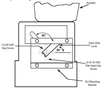
Figure 13. SVI Rotary Mounting Bracket with Valve Side Lever on Ball and Butterfly Valves
