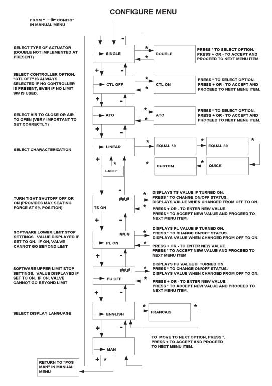
Figure 38. Configure Menu Structures
