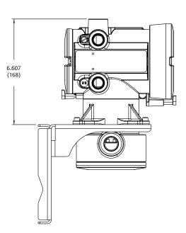
Remote-mount transmitter/core processor assembly with additional conduit opening for installation of the THUM Adapter
