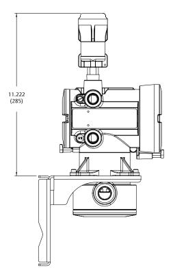
Remote-mount transmitter/core processor assembly with integral-mount THUM Adapter
