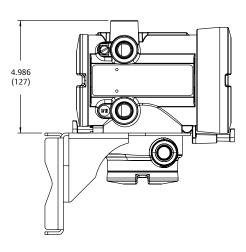
Remote-mount transmitter with additional conduit opening for installation of the THUM Adapter
