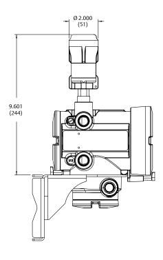
Remote-mount transmitter with integral-mount THUM Adapter
