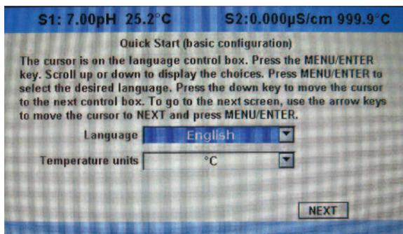
**User Help Screens.** A complete user guide and trouble-shooting manual is embedded in the instrument’s memory and easily accessed via the INFO key on the keypad. Detailed instructions and troubleshooting tips are intended to provide adequate guidance to resolve most problems on site.
