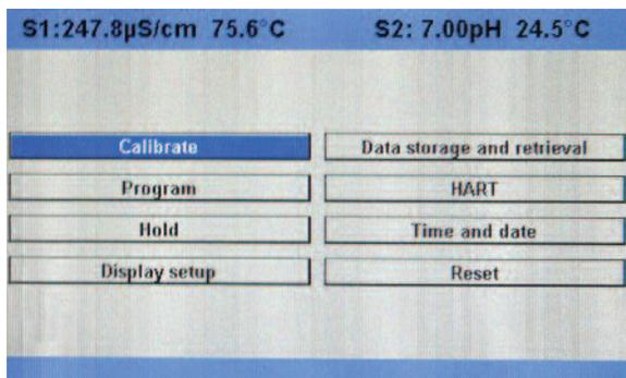
**Quick Start Programming:** Simplified Quick Start screens appear the first time the unit is powered. The instrument auto-recognizes each type of measurement board and prompts the user to configure each sensor loop in a few quick steps for immediate live readings.
