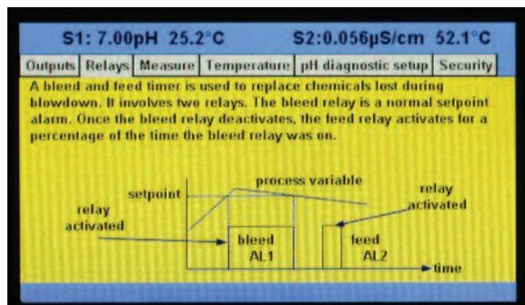
**Timer functions:** Four real-time clock relay functions are implemented including: bleed and feed, day and time interval timers, delay timer and a flow totalizer. These advanced timer features support a number of specialized applications that normally require dedicated timer control devices or DCS programming. Interval timers set relays by interval time, on-time and recovery time for discrete on/off control devices based on measurement inputs.
