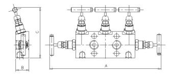
The 'Y53' Type 5 valve manifolds are designed for direct mounting to differential pressure transmitters, with separate isolation and vent for LP and HP inlets plus equalising valve for simple calibration. Each needle valve head is designed for safe and reliable isolation, giving bubble tight shut off, with non-rotating & anti-galling tip and dynamic self-adjusting spindle seal to give long service life in a variety of service conditions.
