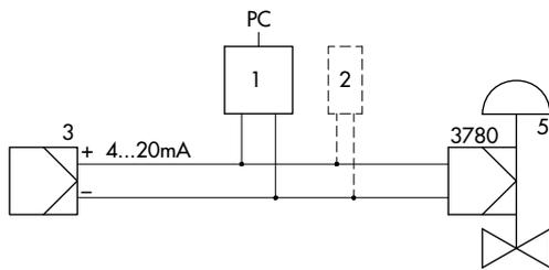
Fig. 7 · Point-to-point communication of Type 3780
