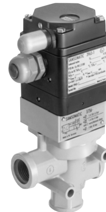
3/2-way solenoid valve, single actuated with spring return mechanism, K_{vs} 4.3, connection G \frac{1}{2}
