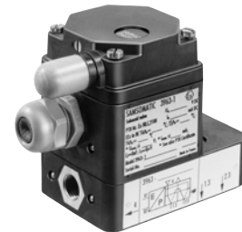
5/2-way solenoid valve, single actuated with spring return mechanism, K_{vs} 0.16, connection G \frac{1}{4}
