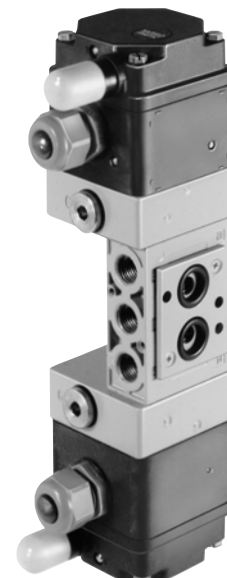
5/2-way solenoid valve, double actuated with two locking positions, K_{vs} 1.4, connection G \frac{1}{4} /NAMUR
