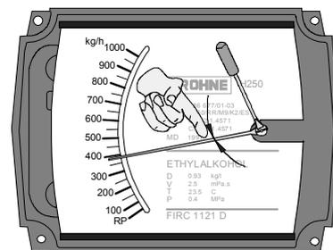
Compare the pointer position with the display value recorded beforehand. If the display value deviates:
