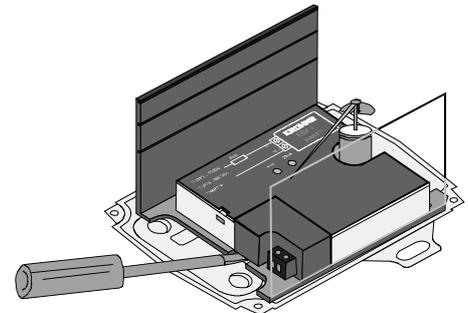
Loosen the locking device of the cover and remove it.
