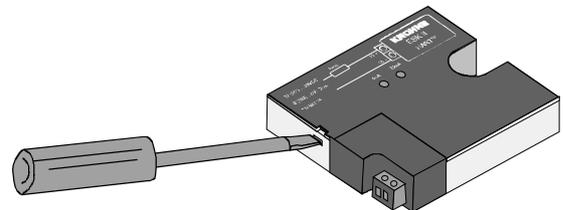
Deformation of the connecting pins can be avoided by lifting the unit at both sides which do not have connections.
