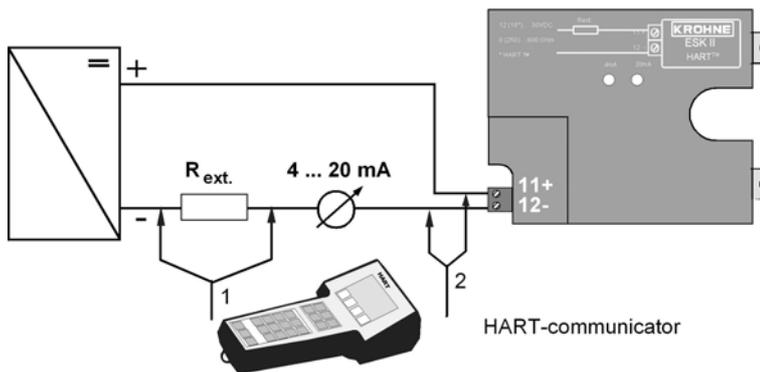
If a HART™ communicator (type Fisher Rosemount, Model 275) or a PC with HART™ modem PC is used, the resistor which is connected in series ( $R_{ext.}$ ) has to exceed 250 Ohms.
