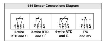
\* Rosemount Inc. provides 4-wire sensors for all single element RTDs. You can use these RTDs in 3-wire configurations by leaving the unneeded leads disconnected and insulated with electrical tape.
